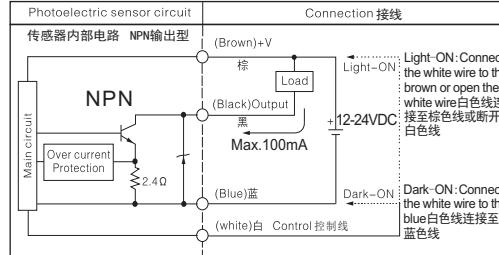
Light ON or Dark ON selectable by control wiring 通过接线(控制线)选择入光ON或遮光ON
